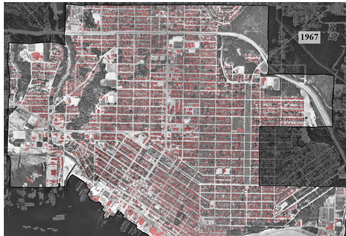
GeoAI example: Buildings extracted from images of 1967 and 2019, North Vancouver, BC
